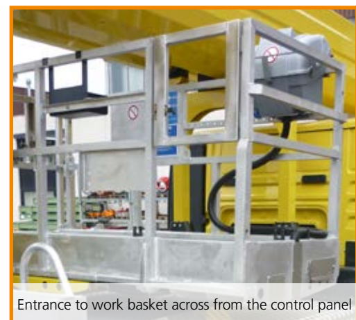
Side entrance to work basket
