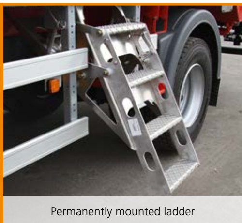
Permanently mounted ladder
