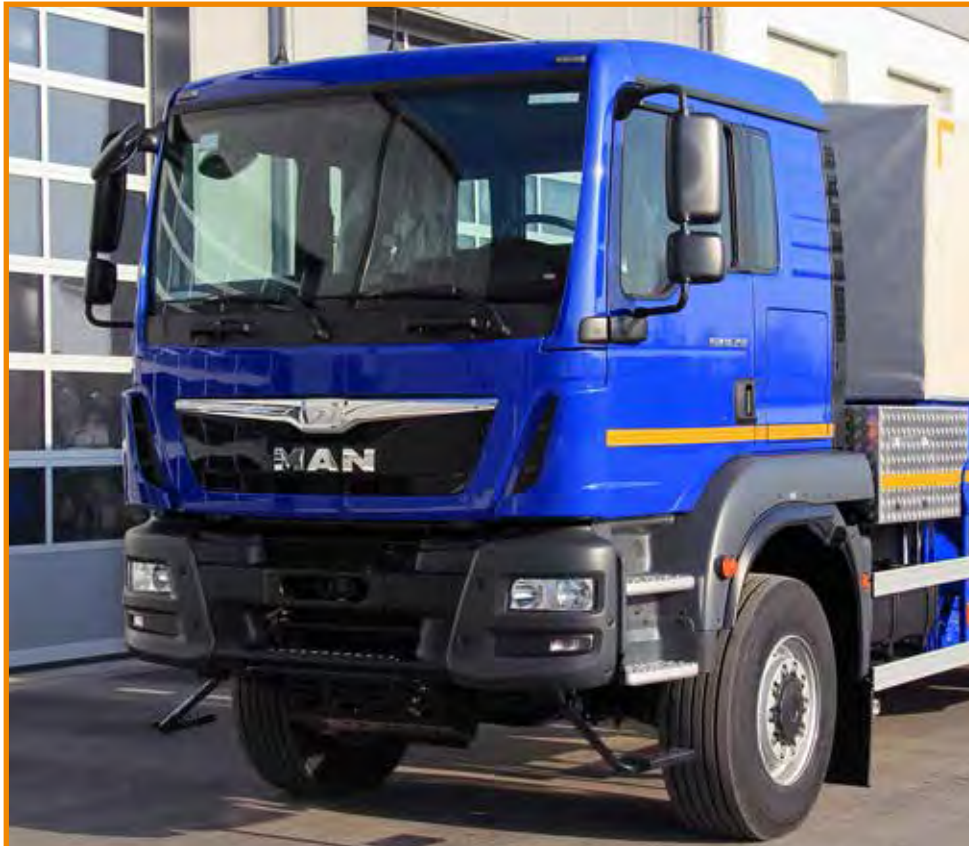
L-cab (seen here on the left) = long sleeper cab for rest and relaxation during down time or additional storage space (storage box, equipment, tools, etc.)
